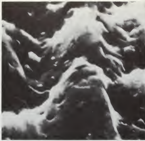
FAST CRACK PROPAGATION (5000X)
